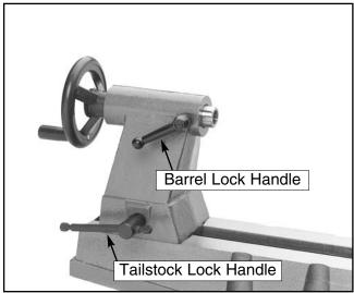
Figure 13. Tailstock assembly.
